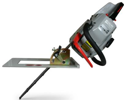
**3. For cuts needing a preset** angle (ex: gang cutting common rafters head cuts) rotate the saw and clamp laterally to the desired angle by loosening and tightening the angle adjustment lever.
